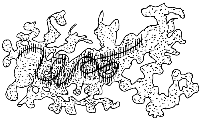
Figure 50. Schematic representation of the MC procedure for simulation of percolation and diffusion together. The shaded region represents parts of the cluster on which diffusion passes, while the dotted areas belong to the cluster but are not constructed by the MC procedure.
