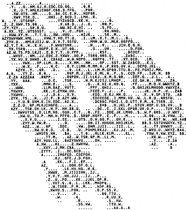
Figure 12. Example of a part of an infinite percolation cluster grown at criticality. The asterisk * is an arbitrary point in the cluster. Sites belonging to shells of successive chemical distance are designated by successive letters of the alphabet (starting with B), and dots designate sites that were tested and found to be empty. The cluster was generated on a triangular lattice, obtained by a square lattice regarding sites along one of the diagonal directions as nearest neighbours.
